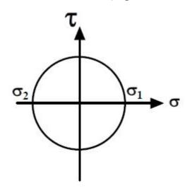
figure- 4.4- Mohr's circle for pure shear
