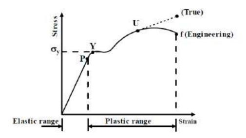
**figure- 3**. (a) Stress-strain diagram for a ductile material e.g. low carbon steel.
