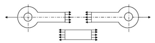
figure-1. - Stresses developed in a link subjected to uniaxial loading
