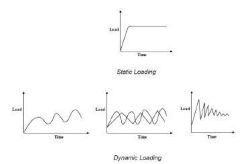
Figure.2 - Types of loading on machine elements.
