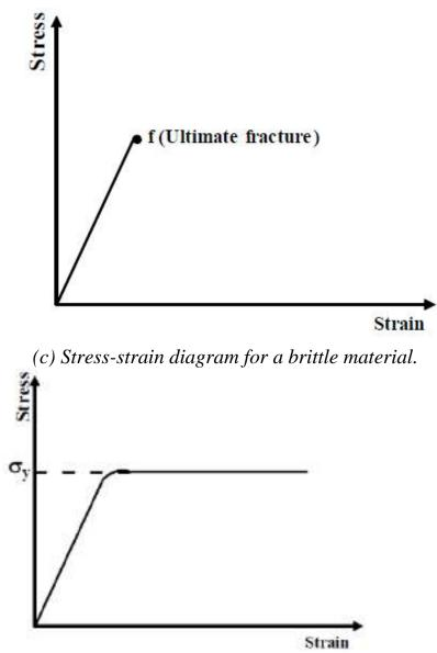
(d) Stress-strain diagram for an elastic – perfectly plastic material.
